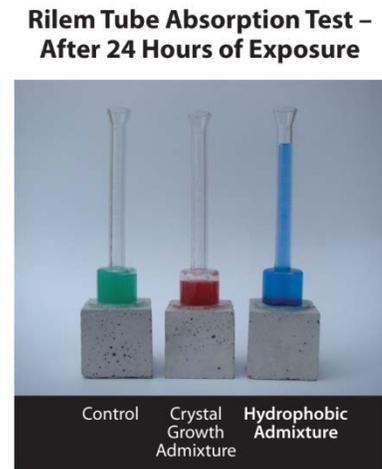
In often repeated studies and experiments, even extremely dense concrete mixes with high compressive strengths, low water cement ratios, and excellent pressure permeability readings rapidly transport water through capillary absorption. To ensure durable concrete it is absolutely essential to adequately address capillary absorption as the designer’s primary duty.
