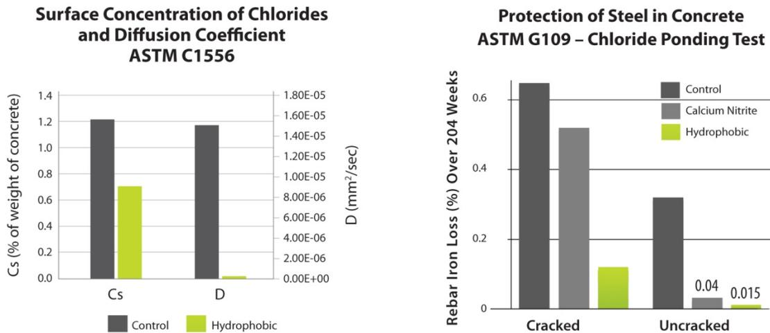
Hydrophobic admixtures reduce both the surface concentration of chlorides in concrete as well as the diffusion coefficient. Also, some hydrophobic admixtures protect steel in both cracked as well as uncracked concrete specimens.
